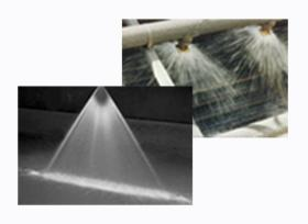
Washdown, coolant, or other liquid spray systems with small orifices can plug quickly.
