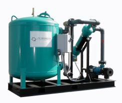
When particulate loads are heavy the requirement for pre-filtration may be necessary to protect finer filtration down stream. Utilizing a *Puroflux* separator as a means of reducing the concentration of solids is a reliable solution that will lower operating and maintenance costs.
